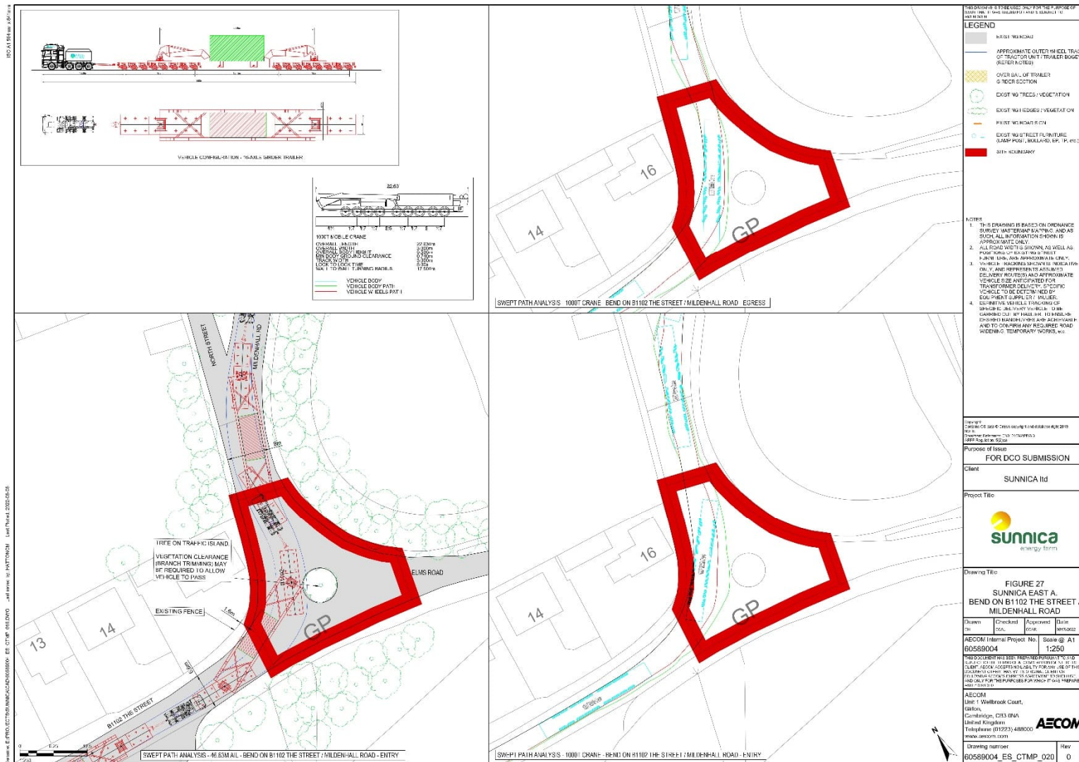
Figure 27: Swept Path Analysis – 1000T Crane and 46.63m AIL – B1102 The Street / Mildenhall Road Junction
